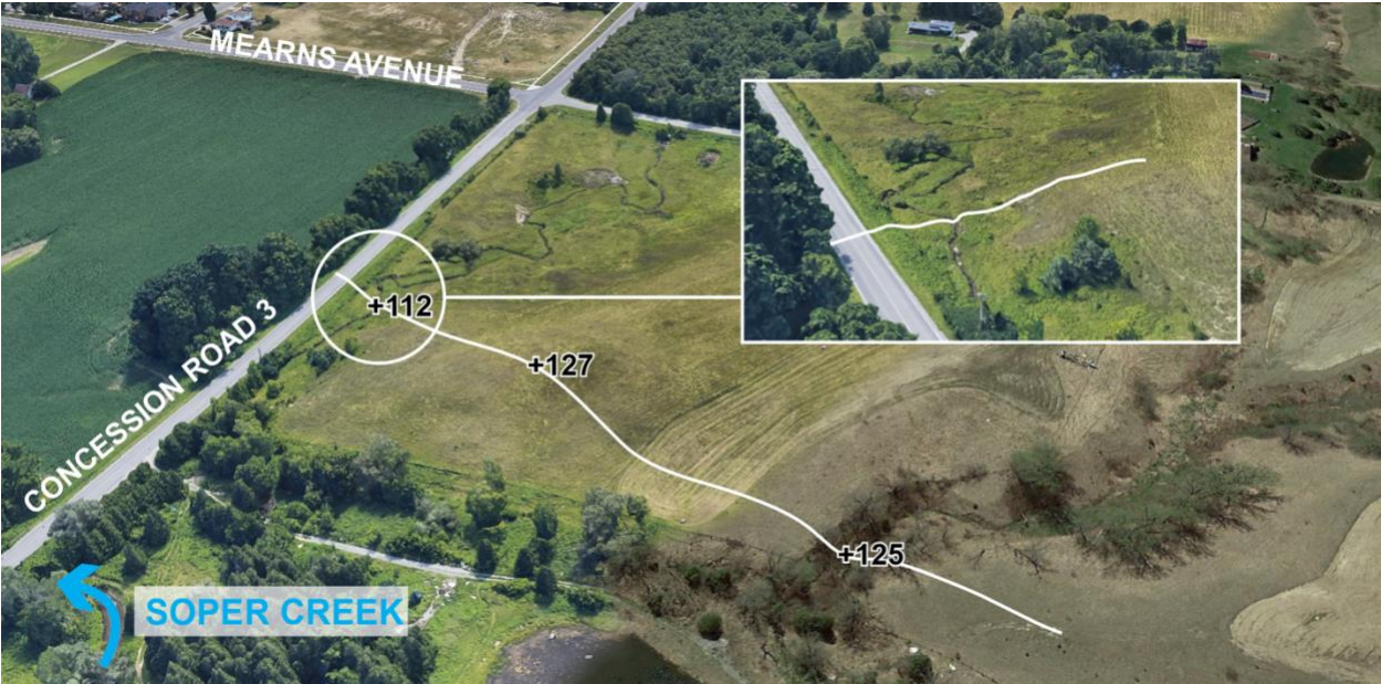
Figure 5: High point (elevation in metres) located in the south of the Study Area, near the corner of Concession Road 3 and Mearns Avenue.
