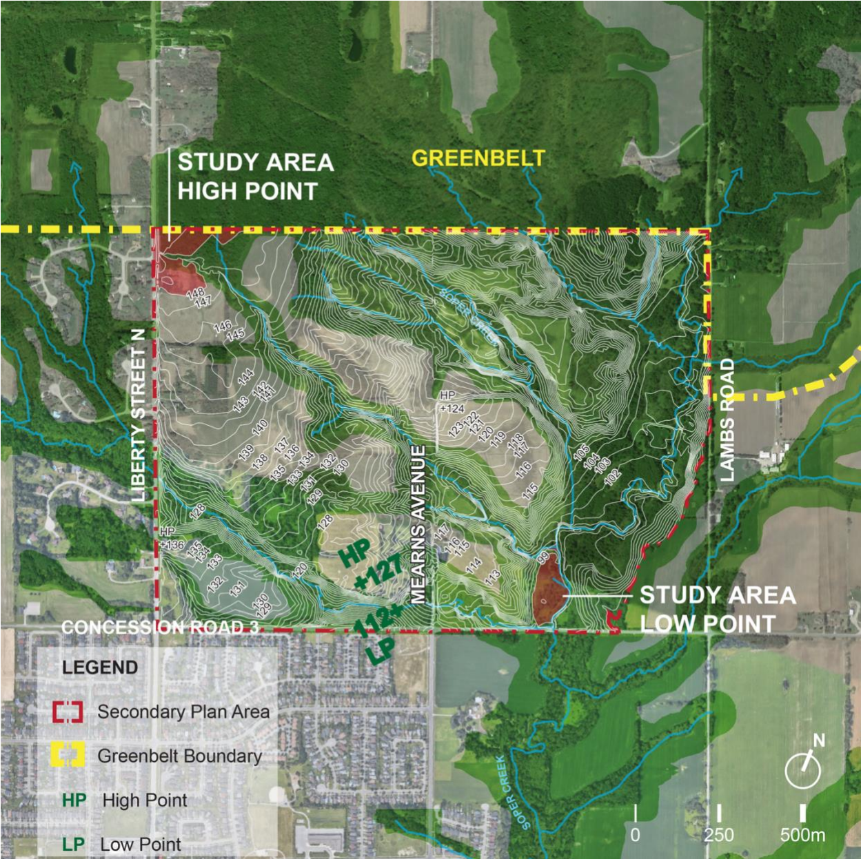
Figure 4: Topographical map of the Soper Springs Secondary Plan Area with 1-meter intervals.
