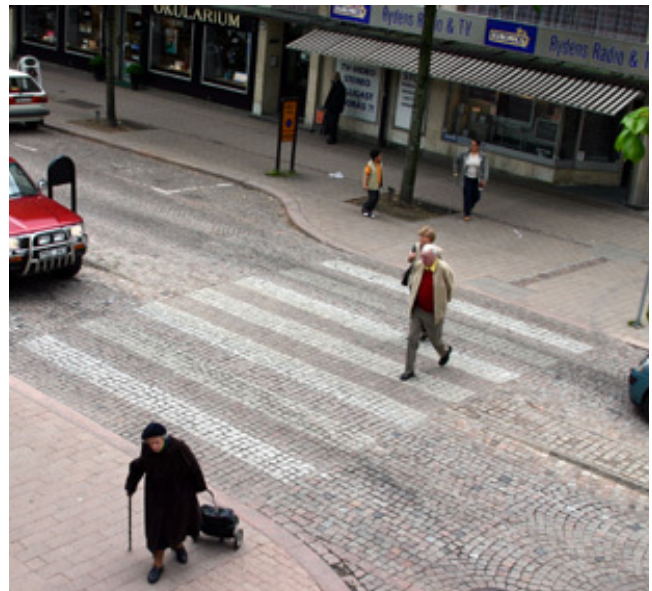
Pedestrian crossings should be identified with distinctive painted lines.
