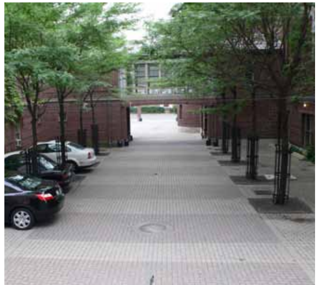
Trees used to break up the parking areas and reduce heat-island effect
