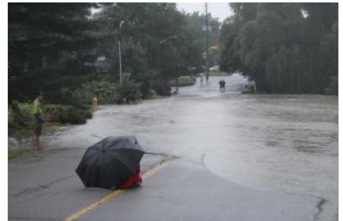
Above: Hard surfaces, such as roadways and parking lots, associated with urban development reduce the amount of water absorbed by vegetation and infiltrated into the soil. The excess runoff can result in an increased risk of flooding. The above photos were taken during a large rainfall event in the Greater Toronto Area in 2013.
